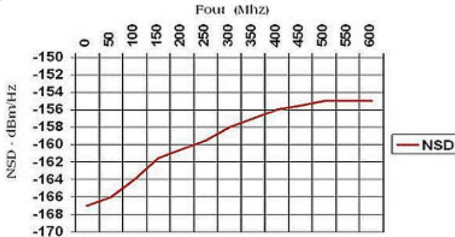
**AD9736 Noise Spectral Density vs Fout at 1.2 GSPS**
