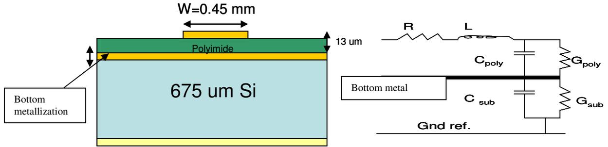
Fig 2: The deposition of metal layer on the bottom of polyimide and its equivalent circuit
