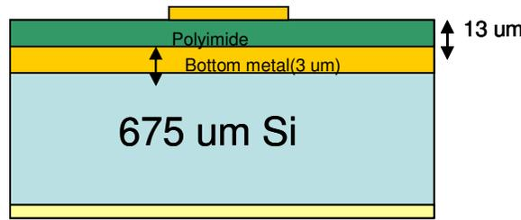
Fig 3: (a) Variation in the bottom metal thickness
