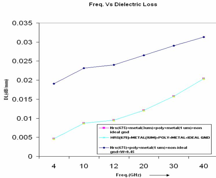
Fig 7: Dielectric Loss variation with frequency [loss comparison with case1]
