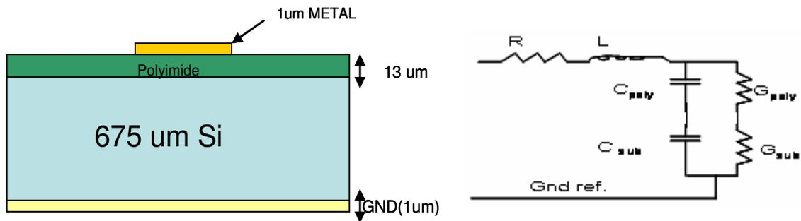
Fig 1: Interface layer of polyimide on Si substrate and equivalent circuit
