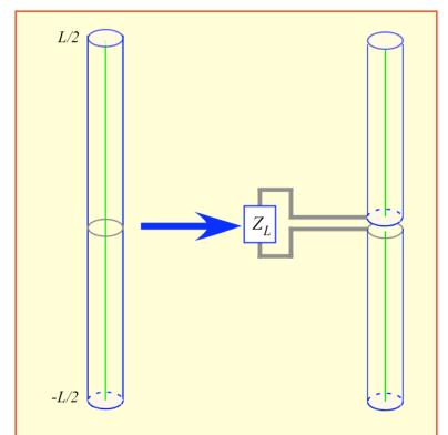
Figure 9: transmission line connected to the two halves of a wire to form a dipole
