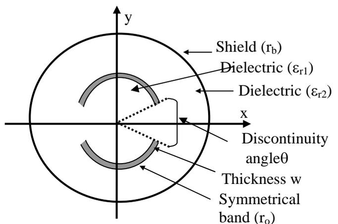
Figure 1 : Cross section of the shielded symmetrical bandline.
