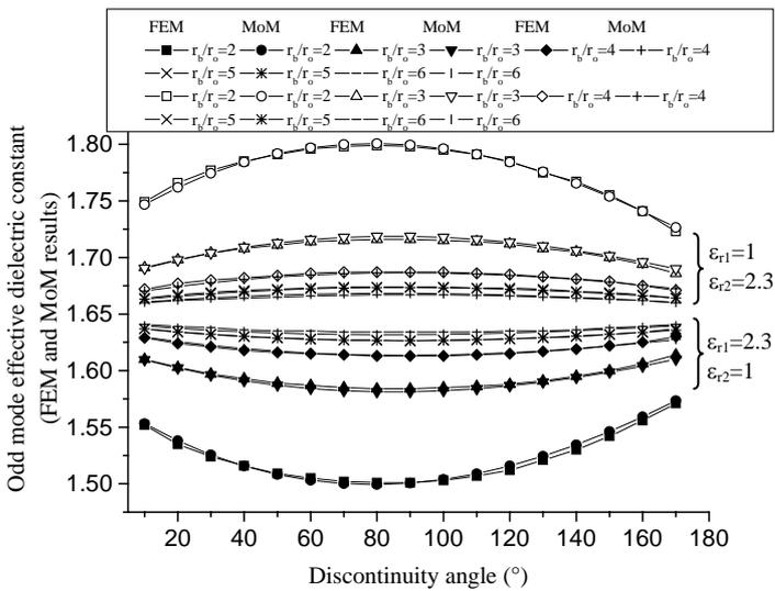
Figure 3 : Effect of the discontinuity angle on the odd mode effective dielectric constant.
