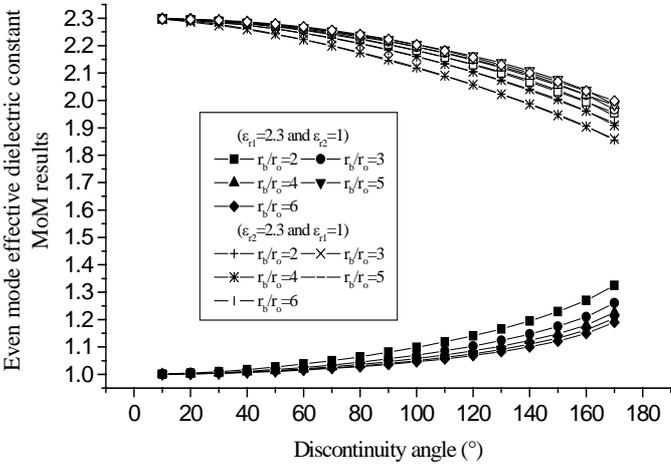
Figure 3 : Effect of the discontinuity angle on the even mode effective dielectric constant using MoM.
