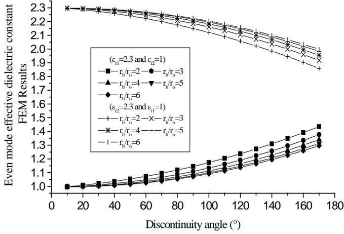
Figure 2 : Effect of the discontinuity angle on the even mode effective dielectric constant using
