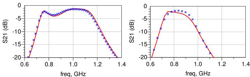
Simulated (lines) and measured (x's) LC-based Band pass filter on 41 mil FR4 (left) and 5 mil FR4 (right).
