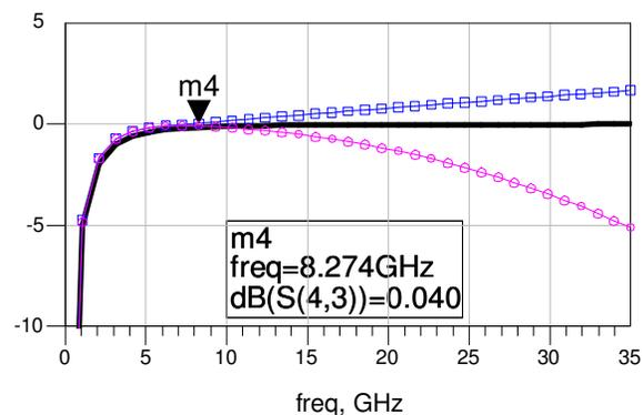
Modelithics Global Models remain well-behaved far above and below the range of measured data used to develop the fitting coefficients for the equivalent circuit model. The model itself is derived from a physically motivated representation of the component. Hence, it does not exhibit non-physical (e.g. gain from a passive component) behavior under extrapolation.
