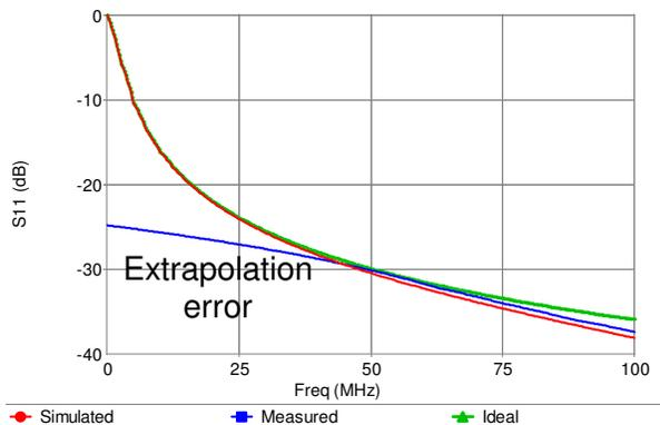
A similar problem can occur when the data is extrapolated below the measured or ideal range, as shown to the left. The model converges to correctly predict the DC response of this capacitor, but when data starting at 50 MHz is extrapolated down to determine the response at a lower
