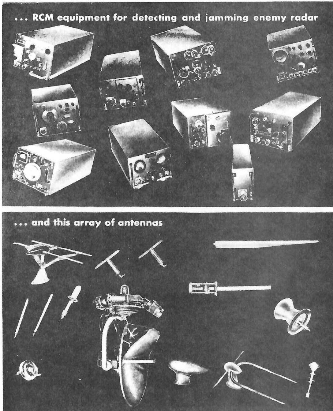
Figure 24b. Most ferret aircraft carried at least four of the RCM (radar counter-measures) equipment, plus all the other equipment shown on these two pages.
