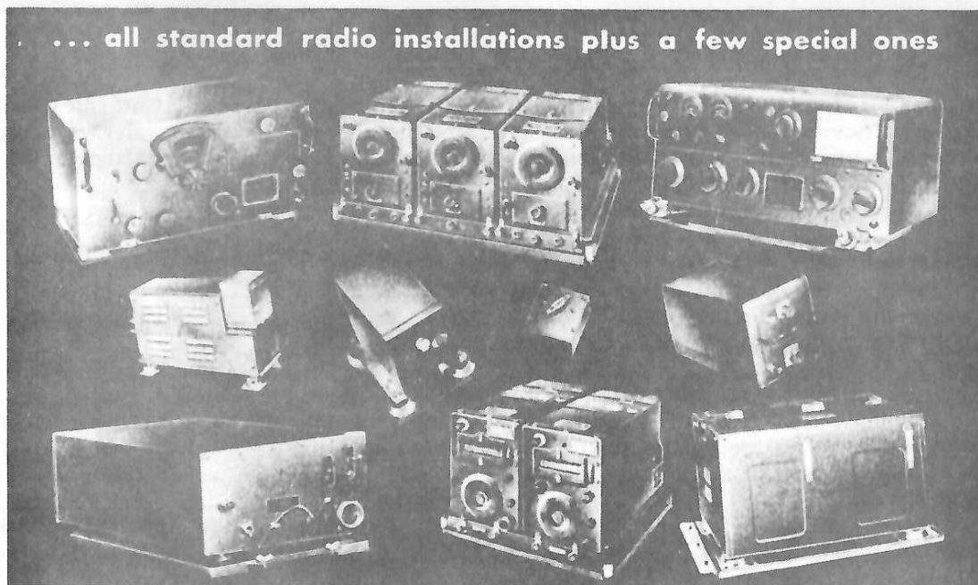
Figure 24a. Electronic equipment for early ferret aircraft. Not shown are power supplies, cabling, control boxes, and numerous other parts.
